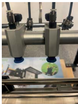
Individual spring-loaded suction elements for optimized sheet separation.
