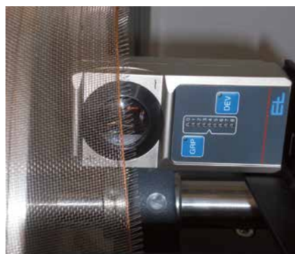
Infrared edge sensor FR 52 for mesh fabric acquisition
