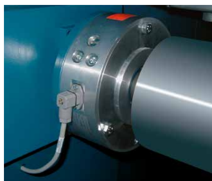
Flange load cell PD 25 on the infeed to a sizing bath
