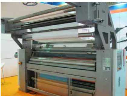
Segmented roller guider system SWS93 on dyeing padder infeed
