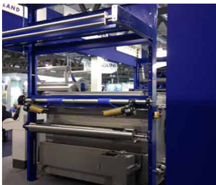
Web guider KF 2020 in the infeed in a textile calender
