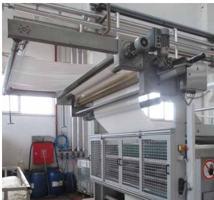
Segmented roller guider system SWS9611 in front of paddler
