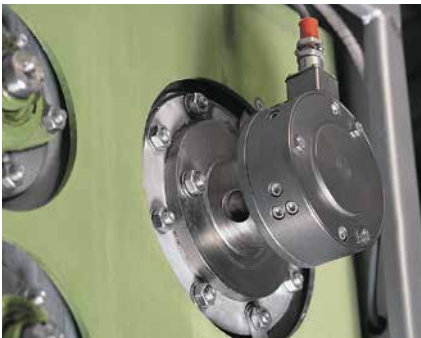
Flange load cell PD 23 on washing machine
