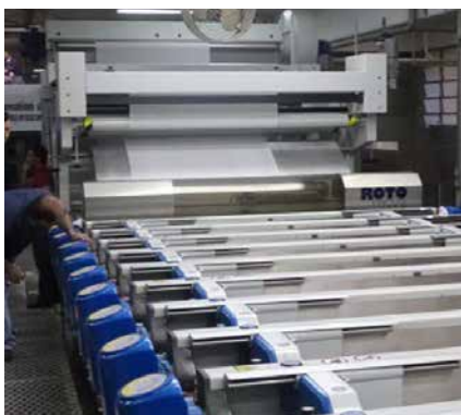
Segmented roller guider system SWS95 on rotary printing machine infeed
