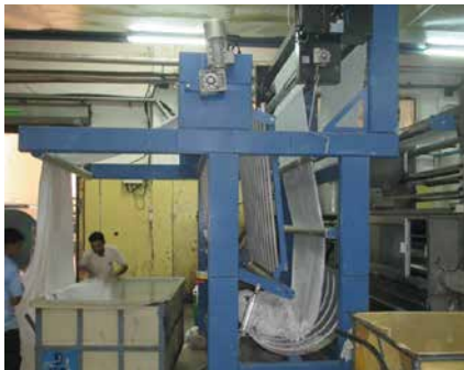
Segmented roller guider system SWA9511 after the J-box before a tenter
