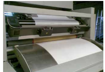
Segmented roller guider system SWS94 on rotary printing machine infeed
